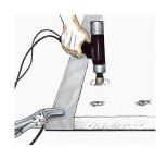
Press the pin through the insulation until the point meets the sheet metal and press the trigger
