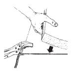
Fix earth clamp of the welder to the sheet metal. Lay insulation on sheet metal
