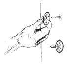
Secure with CL locking washers. If necessary cover the point with a protective cap.
