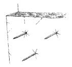
As soon as the strength of adherence is sufficient, impale the insulation on the hangers. Please consult your glue supplierto know about the drying time.
