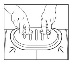
4. Turn straight and pull out slighlty to align. Then tighten knobs.
