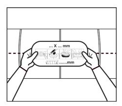
1. Stick self-adhesive template on to duct (a template is provided with each door)
