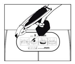
2. Using Turbo Shears or similar cut around template taking care not to exceed the size of the template (the door will function correctly when cut to template size +0 mm -3 mm). For details of the Turbo Shear please refer to Malco Tools Datasheet
