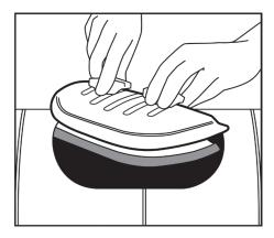
3. Install door by unscrewing the hand knobs until thread is level with top of bolt. Using both hands place the door in the hole at an angle.
